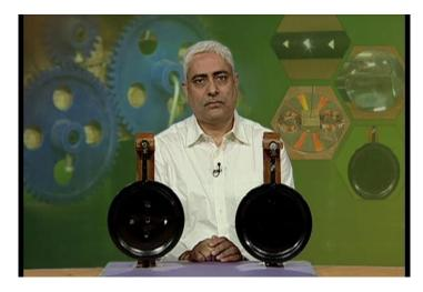
An example of eddy currents is the following: A swinging pendulum, with a conducting sheet, slows down every time it passes through a magnetic field; this 'slowing' is due to the 'eddy currents' induced in the conducting sheet.
