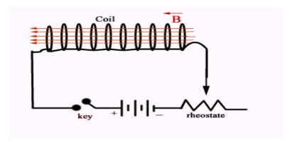
Source: If the current flowing through the circuit is changed by adjusting the rheostat then an emf is self induced in the coil so as to resist this change. As mentioned earlier if I is the current flowing through the coil, the magnetic flux  $(\emptyset)$  linked with the coil is such that:
