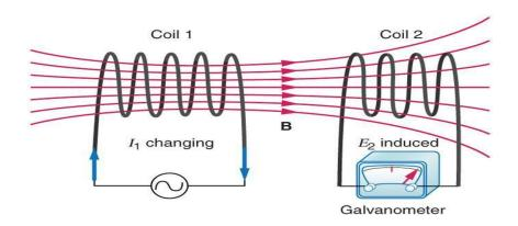
Mutual Induction is a phenomenon in which a changing current in coil 1 produces a changing magnetic flux for coil 2 (placed in its field); this induces an emf in coil 2. This emf is induced in a way so as to oppose the cause of its production.
