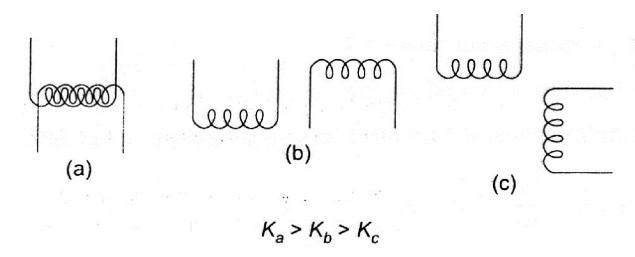
Above Fig. shows a pair of coils in three different orientation, (a), (b), (c), and relative values of their coefficients of coupling. A coil, having some self inductance, is also called an inductor with inductance L.
